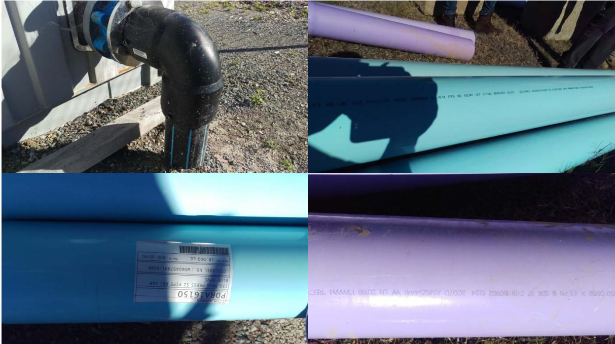
Figure A.5.3 Drinking water and recycled water pipe materials.
